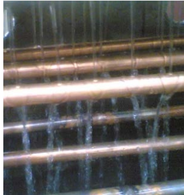
Fig. 3: Falling solution on absorber horizontal tubes
